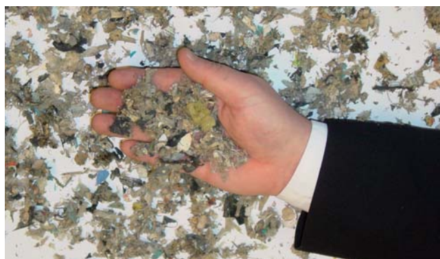
High-quality SRF fuel for the main burner
