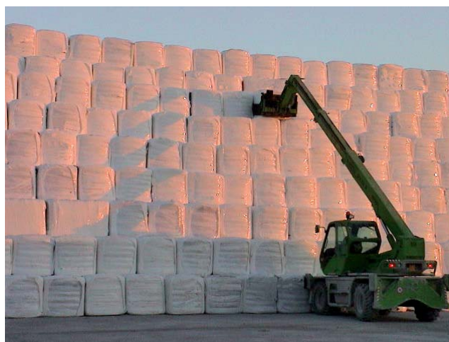
The density of the Energy Cubes is approx. 800 kg/m 3
